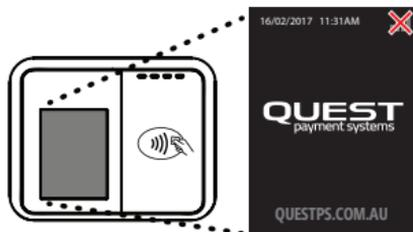
3. Whilst the device is logging onto the 3G network it will display the following image.
